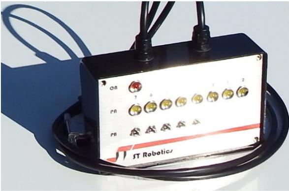
The IO simulator/trainer is a simple device to demonstrate and test I/O from the robot controller.
