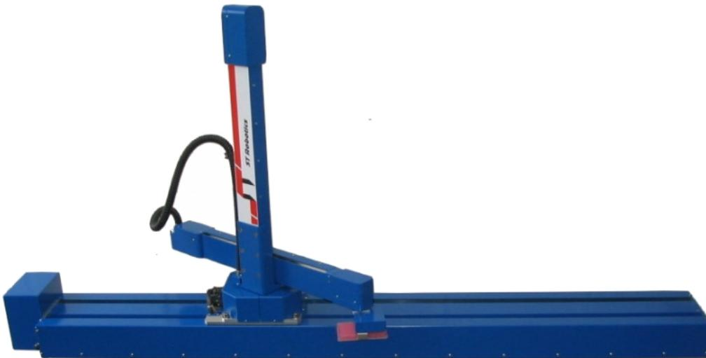
R19 may optionally be mounted on a linear track. This has dual crossed-roller linear bearings providing speed and precision along with smoothness and lack of vibration and noise. Max speed 1000mm/sec. Positional repeatability 0.2mm. R19D pictured on 1m track. High speed version available.
