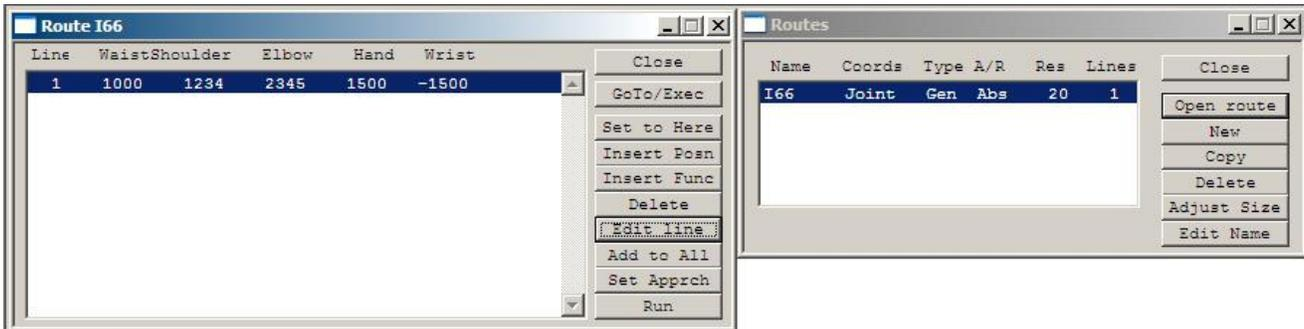
For the next position highlight the next blank line and click **Insert Posn** again. Don't forget to click back inside the communications window before you type a command.
