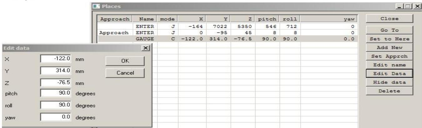
The screenshot shows the 'Places' window with a table of place data. The table has columns for Approach, Name, mode, X, Y, Z, pitch, roll, and yaw. The 'GAUGE' row is highlighted. An 'Edit data' dialog box is open, showing input fields for X, Y, Z, pitch, roll, and yaw, with units (mm or degrees) and OK/Cancel buttons.
