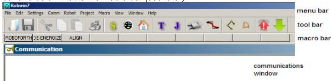
**Load/check settings:** On the menu bar click settings, open file. If you have an R12 or R17 click on r12r17.cfg; if an R19 click on R19.CFG. Axis names may be manually set using settings **caps lock** – All ROBOFORTH commands are in upper case, ensure CAPS LOCK is on.
