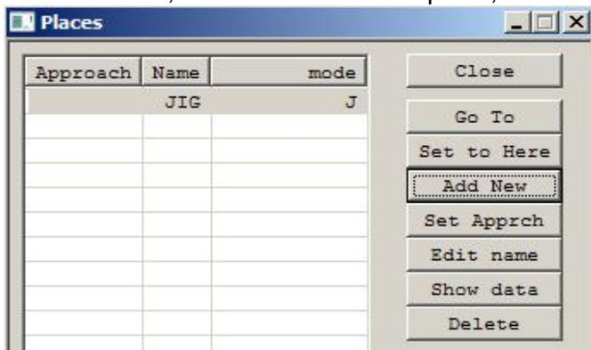
To make the robot move to this position click the communications window and enter the name of the place, for example suppose the place name were JIG. Enter:
